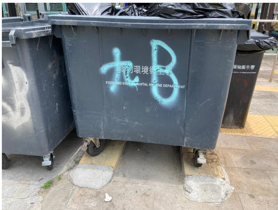
Figure 3.10. A “660” wheelie bin mounted on concrete steps for easy transfer onto a more maneuverable hand cart. 660s are loaded sideways onto trolleys for easier transportation by a single worker.
